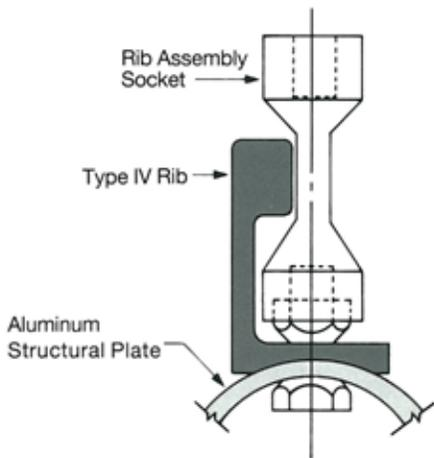
The socket is specially shaped to fit around the top “bulb” of the reinforcing rib. This is a six-point socket for 1-1/4” nuts and with a 3/4” drive. This socket will work on both Type II and Type IV ribs. Contech offers this socket as a construction aid.
